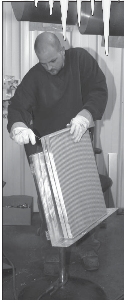
Brad Richardt begins the labor-intensive process by deburring the core. After he finishes, there are nine additional steps before the finished radiator goes into the box and is shipped.
